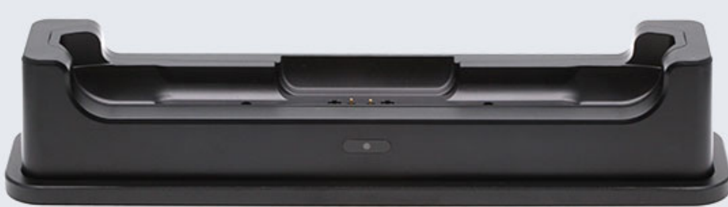
CRD-P80-RBC Charging Cradle for device, use with DCPWR-5V2A-(CN/EU/UK/US) adaptor and TYPE C cable. The cradle cup has an insert that is fixed by 4 pcs screws and they must be removed in prior when charging P80 with rugged boot.
