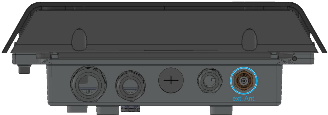
Fig. 6: External antenna connection
