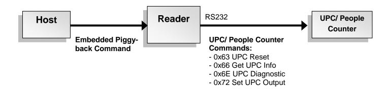
Fig. 1: Communication of a system consisting of a Host, Reader and UPC/ People Counte
