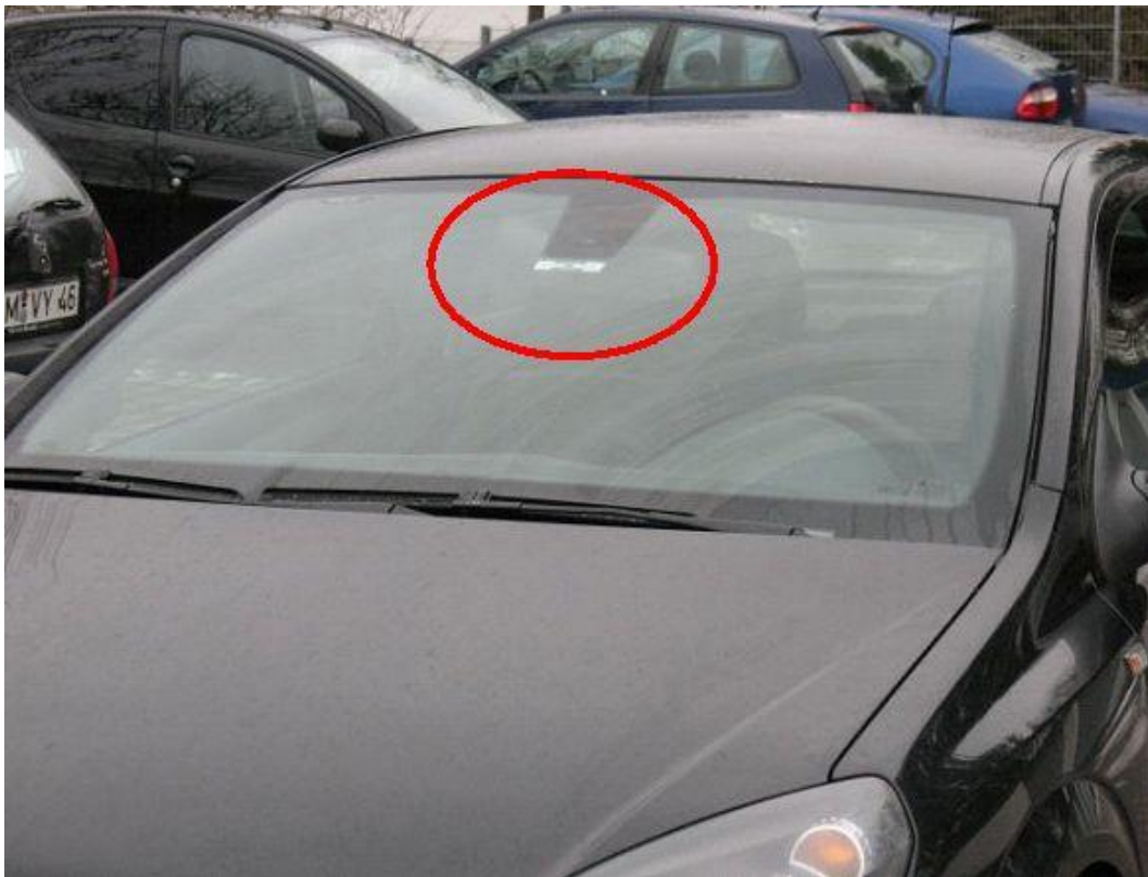
Figure 19: Mounting of the transponder
