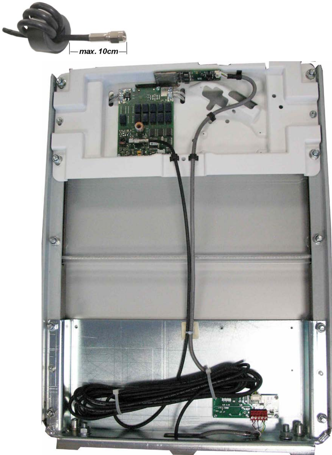
Fig. 20: Unused coaxial cables are tied in antenna Type B
