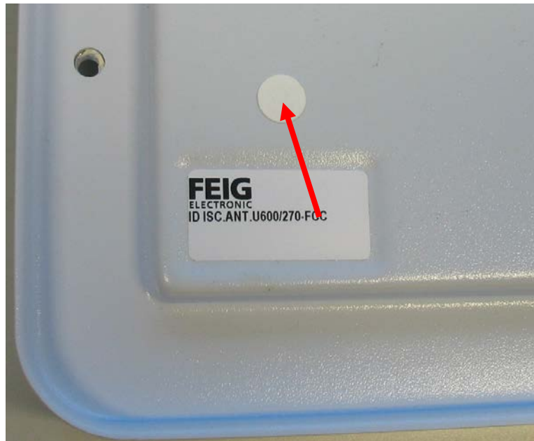
Figure 4: Membrane for pressure balance
