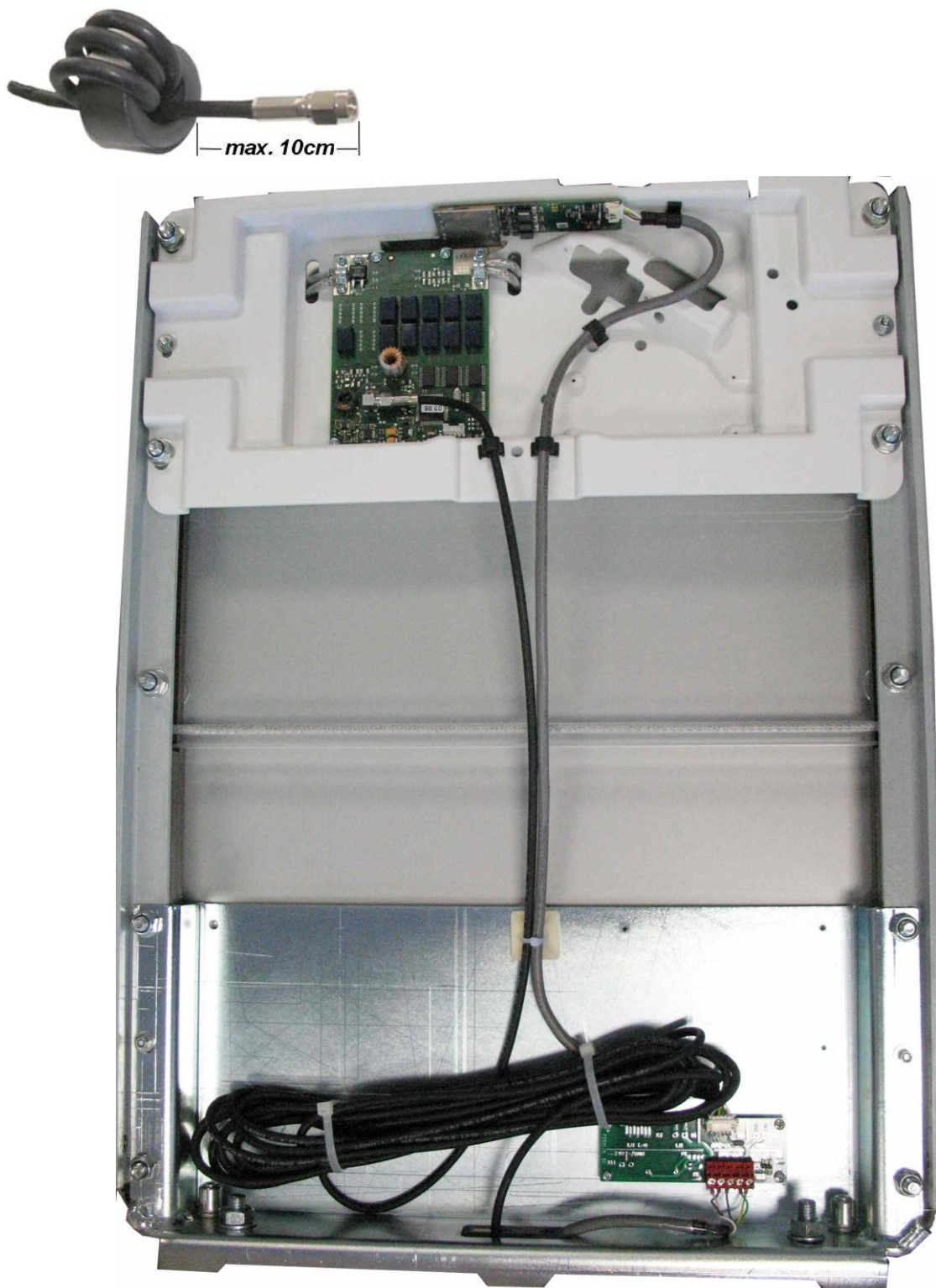
Fig. 21: Unused coaxial cables are tied in antenna Type B
