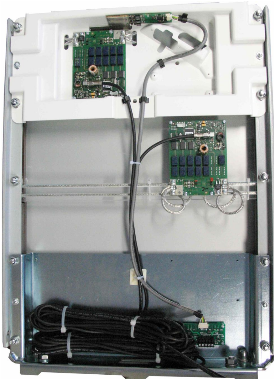
Fig. 20: Unused coaxial cables must be fixed in antenna Type B
