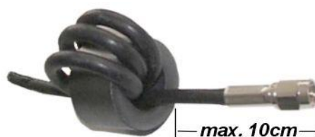
Figure 3: Antenna line with EMC ring cores
