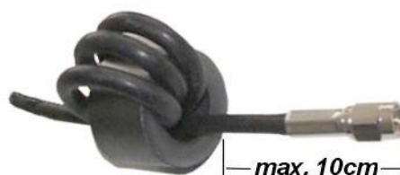
Figure 5: Antenna line with EMC ring cores
