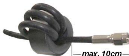
Figure 3: Antenna line with EMC ring cores
