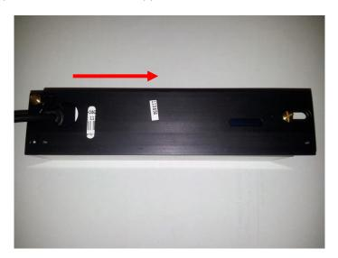
Two brass screws should not be loosening. If these two screws are loosed, the slot where the card is swiped can move, changing the pressure and the space by the cards.
